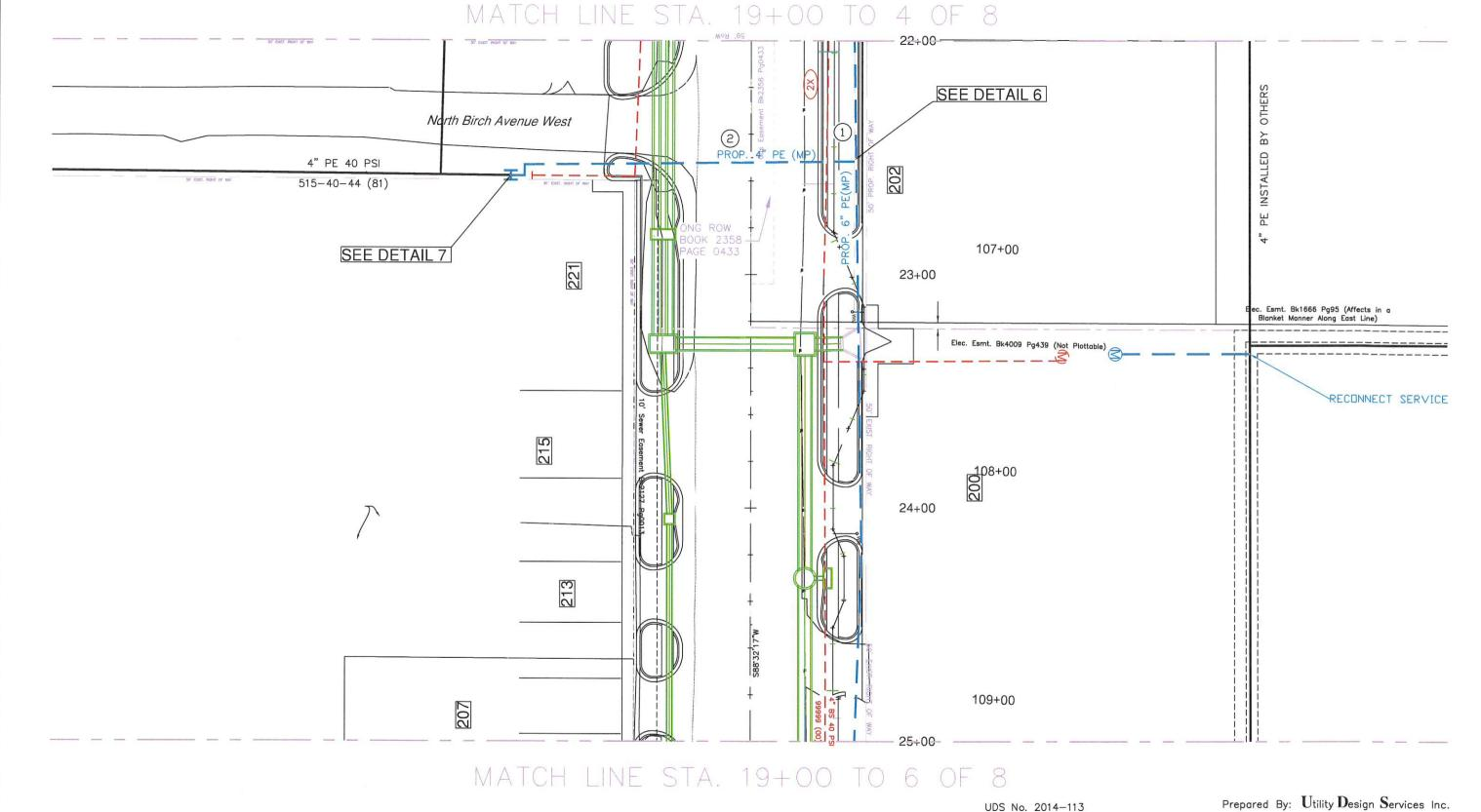
MAINTAIN 5' HORIZONTAL SEPARATION AND 2' VERTICAL SEPARATION OF ALL WATERLINES
