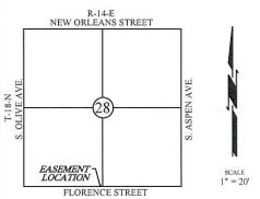
BASIS OF BEARING FOR THIS SURVEY IS THE SOUTH LINE OF THE SW/4 OF SECTION 28 BEING S 88°34'42"W
