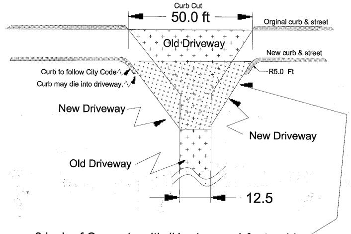
6 inch of Concrete with #4 rebar on 1 foot grid
