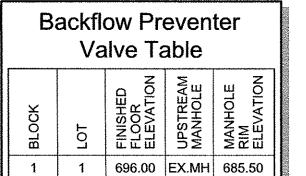
FINISHED FLOOR ELEVATION SHALL BE 1'-0" ABOVE FINISHED PAD ELEVATION. IF THE ACTUAL FINISH FLOOR ELEVATION IS LOWER THAN ONE (1) FOOT ABOVE THE TOP OF RIM ELEVATION OF THE UPSTREAM MANHOLE, IT SHALL BE THE BUILDER'S RESPONSIBILITY TO INSTALL A BACKFLOW PREVENTER VALVE NEAR THE BUILDING ACCORDING TO BROKEN ARROW ORDINANCE NO. 1777, SECTION
