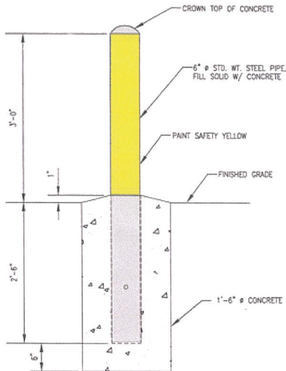
Steel Bollard Detail
