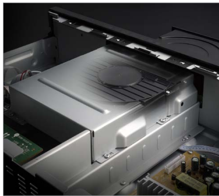
Fully Shielded Mechanism
