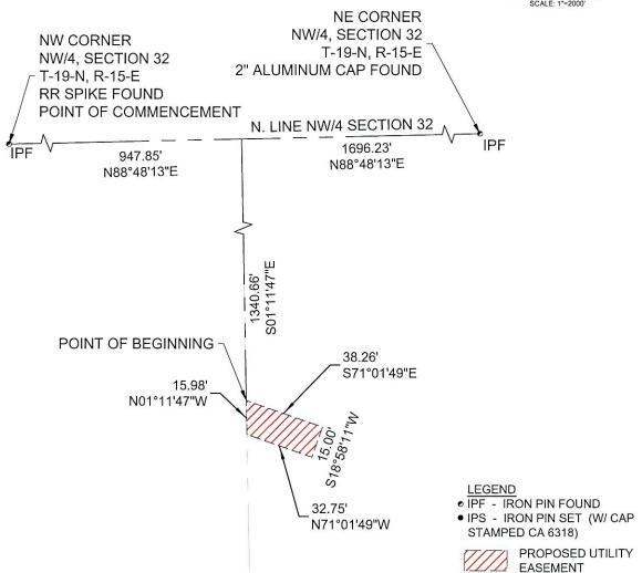
BASIS OF BEARINGS IS THE OKLAHOMA STATE PLANE COORDINATE SYSTEM (ZONE 3501 NORTH) WITH THE NORTH LINE OF NW/4 BEING N 88°48'13" E.
