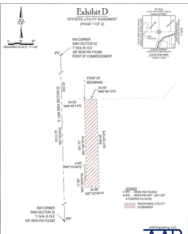
BASIS OF BEARINGS IS THE OKLAHOMA STATE PLANE COORDINATE SYSTEM (ZONE 3501 NORTH) WITH THE EAST LINE OF SW/4 BEING S 01°29'16" E.
