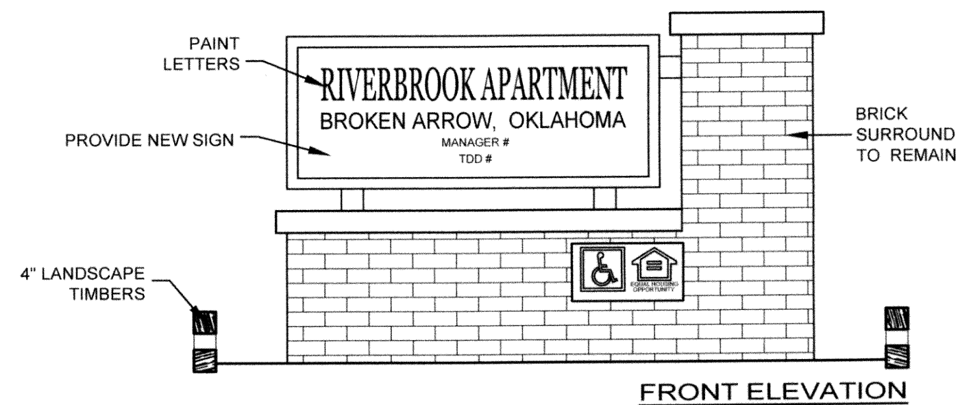
1002 PROJECT SIGN DETAIL SCALE: 1/2" = 1'-0"
