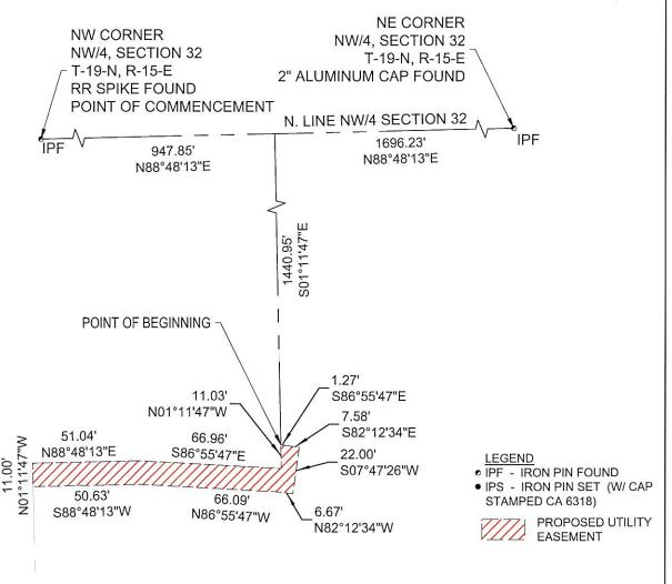
BASIS OF BEARINGS IS THE OKLAHOMA STATE PLANE COORDINATE SYSTEM (ZONE 3501 NORTH) WITH THE NORTH LINE OF NW/4 BEING N 88°48'13" E.
