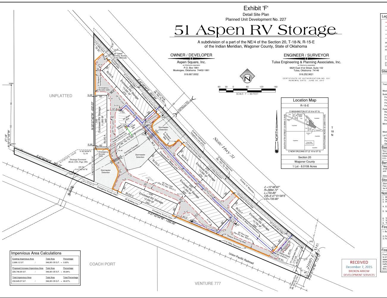
Legend = Light Pole SSMH = Sanitary Sewer Manhole Fire Hydrant STMH = Storm Sewer Manhole 20' Fire Lane (Per IFC 503.3, 503.7.2.1, 503.7.3.3, Appendix D and City Ordinance 3313.4)
