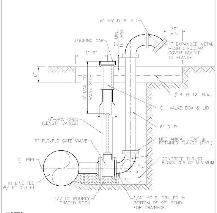
1. ALL EXPOSED METAL TO RECEIVE 2 COATS OF ALUMINUM INDUSTRIAL GRADE PAINT. CONCRETE PAD TO BE 2' - 8" X 8" X 8"
