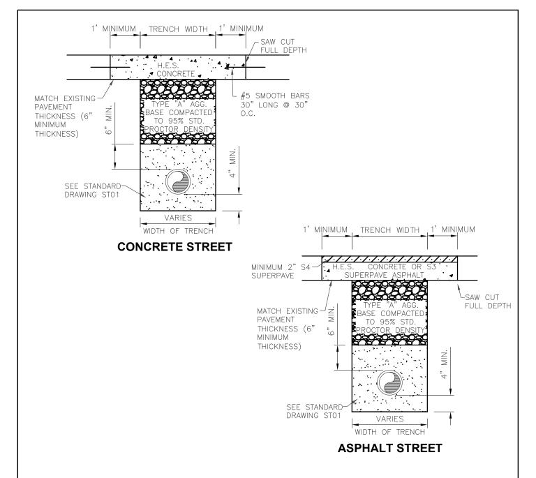
USE THIS DETAIL WHERE IT IS NECESSARY TO CUT THE PRESENT SURFACE FOR REMOVAL OR CONSTRUCTION OF AN UNDERGROUND FACILITY
