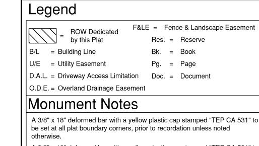
A 3/8" x 18" deformed bar with a yellow plastic cap stamped "TEP CA 531" to be set at all lot corners after completion of improvements, unless noted
