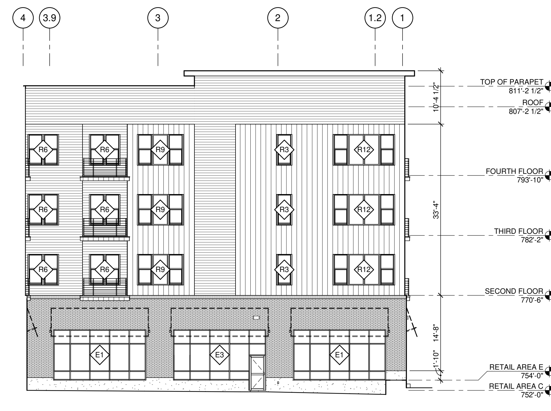
3 SOUTH WING NORTH ELEVATION 3/32" = 1'-0"
