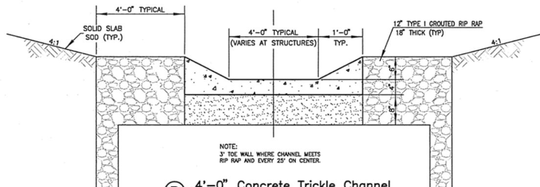
**B 4'-0" Concrete Trickle Channel**
