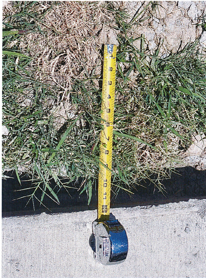
Figure 21: No excavation 1 foot past curb
