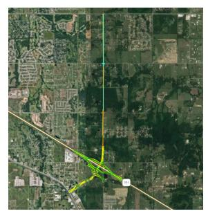
This project will construct a new connector roadway between State Highway (SH)-51 and the proposed interchange with the Muskogee Turnpike and widen and reconstruct a 3-mile section of 273rd E. Avenue north of the Muskogee Turnpike. The Project involves three independent components.
