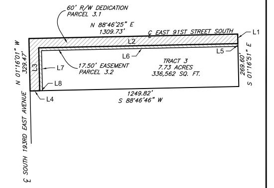
THE BEARINGS SHOWN HEREON ARE BASED ON THE OKLAHOMA STATE PLANE COORDINATE SYSTEM NAD 83 (2011) AND THE WEST LINE OF THE NW/4 BEING NORTH 01'16'01" WEST.
