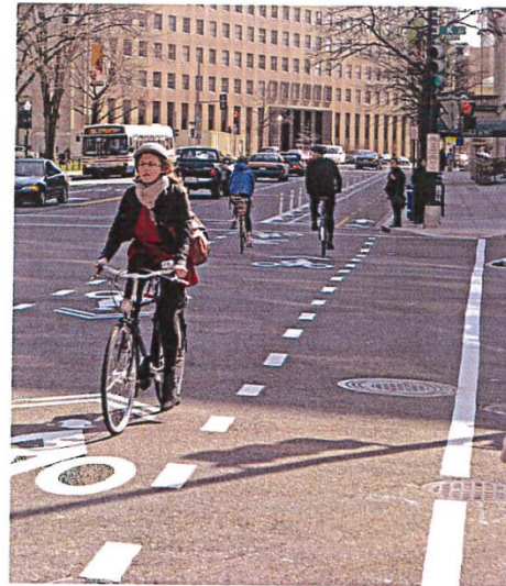
Striping bike facilities through intersections highlights the bicyclist's path of travel
